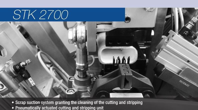
Electro-mechanic crimping system optionally implemented with CFM
